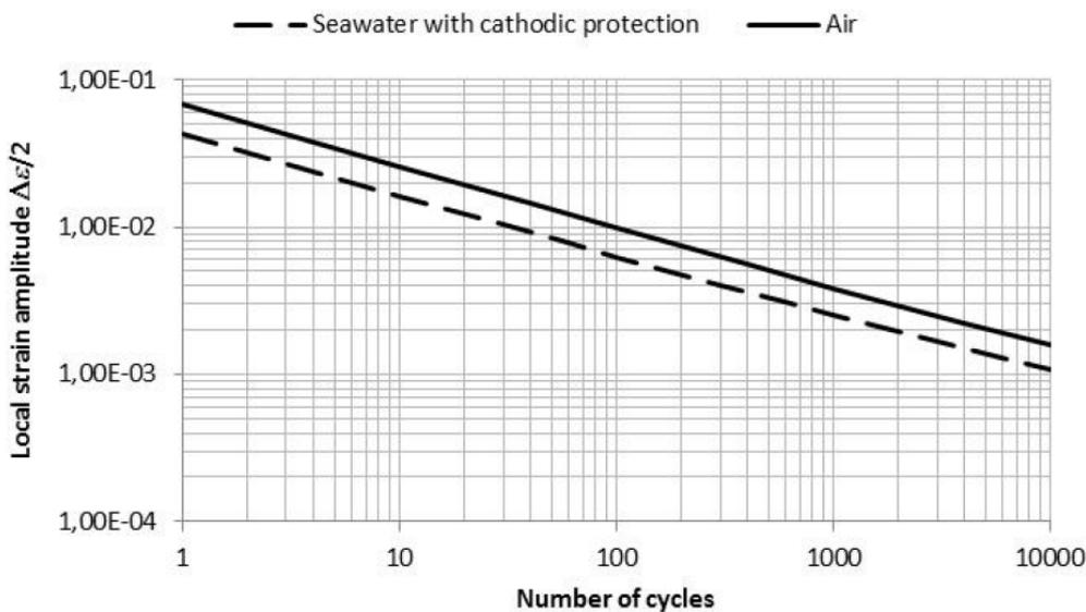
A limitation of RP-C208 is that it only covers steel grades S235, S355, S420 and S460. So the extra high steel grades with yield stresses between 500-700 N/mm<sup>2</sup>, which are increasingly used in high loaded steel structures, are not described. However, with lack of availability of further data (and an apparent soft relationship between allowable strain and yield stress), above curve can also be carefully used for extra high steel grades.
